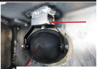
NOTE: Bolt and spring washer only from light side with nut to top
